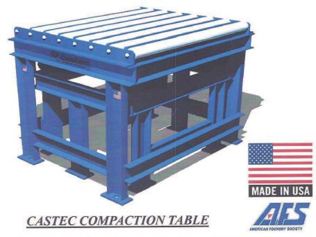
Compaction Tables are used to increase the efficiency and consistency of making quality Molds and Cores. Compaction Tables can also reduce "burn-in" which results in reduced binder levels and less time in the cleaning room.
